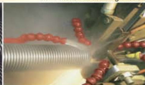
Continuous Fin Welding Process
